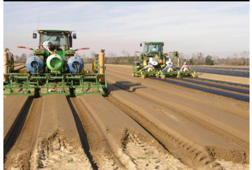
Fig 2. Knives mounted to second bed press to inject metam sodium followed by plastic layer.
